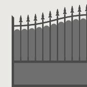
TÔLAGE AVEC FESTONNAGE SUIVANT FORME
